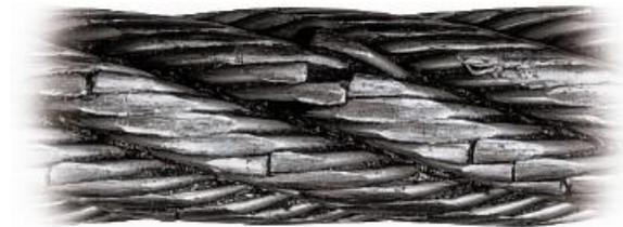
A typical failure of a rotary drill line with a poor cutoff practice. These wires have been subjected to continued peening, causing fatigue type failures. A predetermined, regularly scheduled cutoff practice can help eliminate this type of problem.
