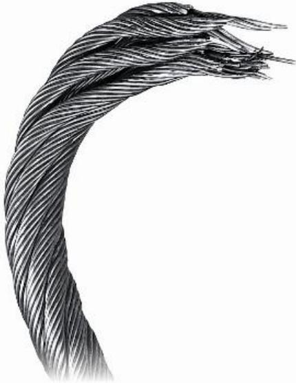
Here's a wire rope that has jumped a sheave. The rope "curled" as it went over the edge of the sheave. When you study the wires, you'll see two types of breaks here: tensile "cup and cone" breaks and shear breaks that appear to have been cut on an angle.
