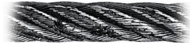
This is localized wear over an equalized sheave. The danger here is that it's invisible during the rope's operation, and that's why you need to inspect this portion of an operating rope regularly. The rope should be pulled off the sheave during inspection and bent to check for broken wires.
