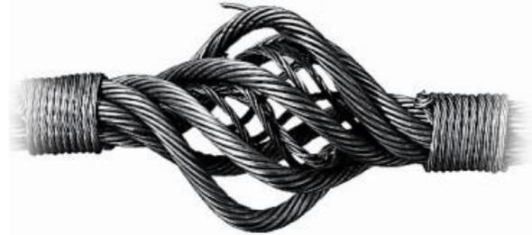
A “birdcage” is caused by sudden release of tension and the resulting rebound of rope. These strands and wires will not be returned to their original positions. The rope should be replaced immediately.
