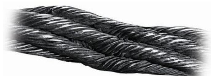
This is a wire that has been kinked. It's caused by pulling down a loop in a slack line during handling, installation or operation. Note the distortion of the strands and individual wires. This rope must be replaced.
