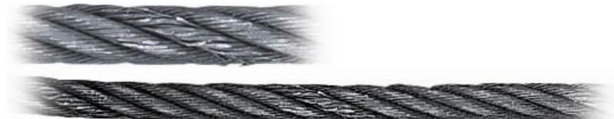
This is a wire rope with a high strand— a condition in which one or more strands are worn before adjoining strands. This is caused by improper socketing or seizing, kinks or dog-legs. At top, you see a closeup of the concentration of wear. At bottom, you see how it recurs every sixth strand in a 6 strand rope.
